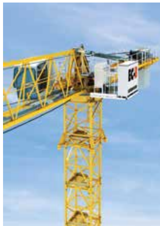
The new tower crane has 15 percent better capacities and can now lift 2,100kg at its maximum radius of 60 metres.
