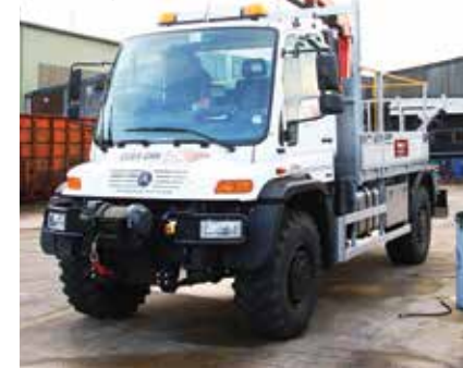
A Unimog mounted Palfinger PK 10002 SH for UK Power Networks at the Devizes depot.
