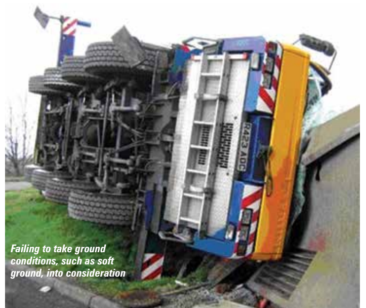
A consequence of programming in the wrong counterweight and deviating from plan
