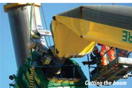
Boom removed and draining all the oil into the telehandler mounted plastic container
