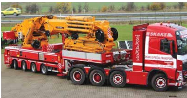
The crane is mounted on a four axle trailer pulled by four axle tractor unit. The unit travels fully rigged.
