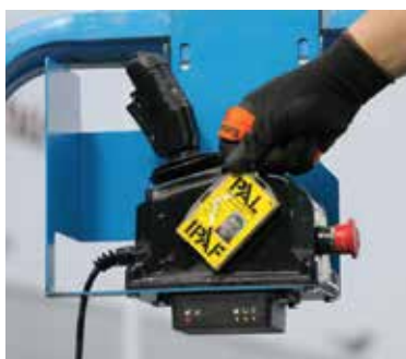
IPAF's new Smart PAL can be used to prevent untrained operation as well as fraudulent use.
