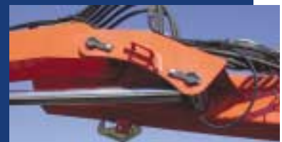
Linkages and pins between booms
