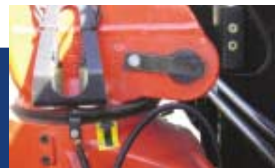
Column around base and ram pivot
