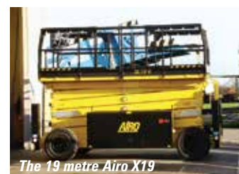
Airo uses a larger central section scissor stack
