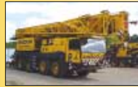
Liebherr LTM1090/2 Year 1997. Capacity 90 tonnes. All Terrain
