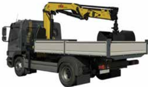
The Hyva HC K series with double linkages, designed for heavy duty deliveries, such as grab and clamshell work
