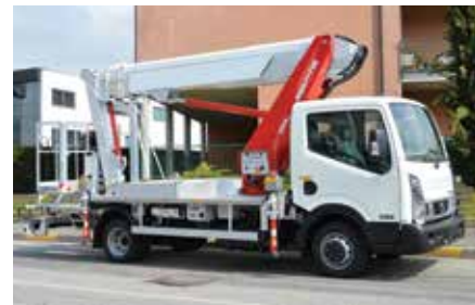
The new 22.6 metre MJ 226 features a telescopic boom plus telescopic articulating jib.
