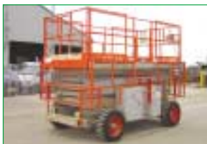
SELF PROPELLED SCISSOR 1997 SKYJACK 8841 14m. working height (47ft.). 2WD, Twin Extending Decks.
