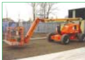
SELF PROPELLED TELESCOPIC 2002 JLG 600AJ 18m. working height (60ft.) 4WD, Articulated Boom.
