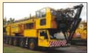
Spierings SK598 Year 2003. Capacity 8 tonnes. Mobile Tower
