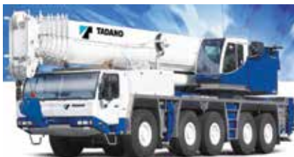
Tadano's new 220G-5 with telescopic luffing jib.
