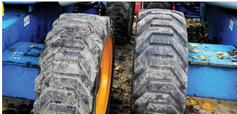
A Niftylift boom with non-marking tread on top of a standard black carcass
