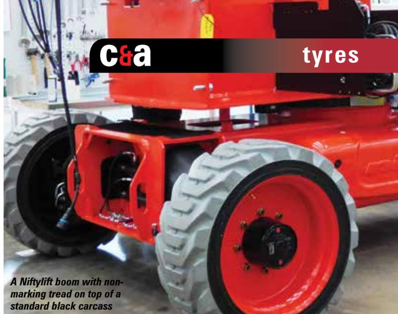
A Niftylift boom with non-marking tread on top of a standard black carcass
