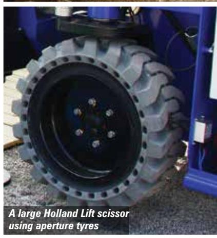
*A large Holland Lift scissor using aperture tyres*
