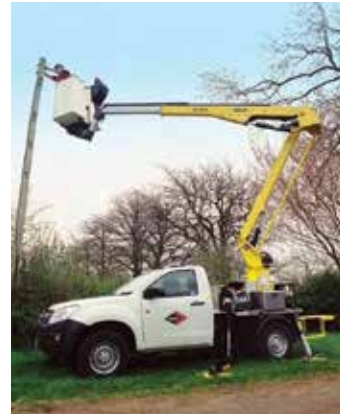
Versalift's 13.3 metre LAT135-H platform incorporates certified low voltage - 1kV AC - insulation to European LV standard VDE 0682-742
