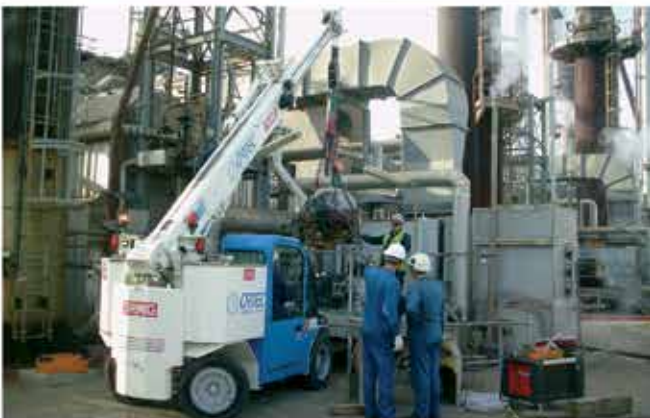
The five tonne MPK50 has a maximum lift height of eight metres
