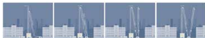
The Mammoet Focus can self-erect in the vertical plane.
