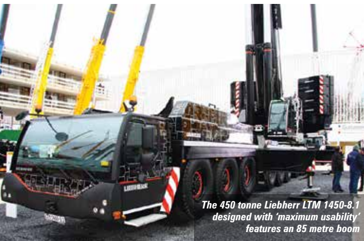
One of the LTM 1450s distinctive features is its variable hydraulically adjustable counterweight radius
