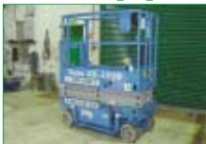
SELF PROPELLED SCISSOR 2002 GENIE GS1930 7.6m Working Height (25ft) Compact Design, Slide-out Deck
