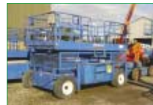
SELF PROPELLED SCISSOR 2000 UPRIGHT LX41 4X4 14.3m. working height (47ft.). Kubota diesel, dual deck extensions.
