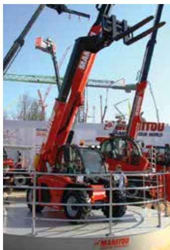
The two tonne/4.28 metre sub-compact MT420 H which has an overall width of 1.49 metres, and an overall height of 1.9 metres
