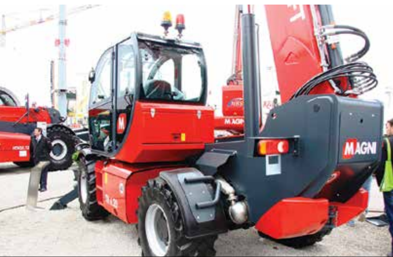
Magni has also launched a new range of regular straight frame machines starting with the six tonne capacity TH 6.20 with a 19.2 metre lift height
