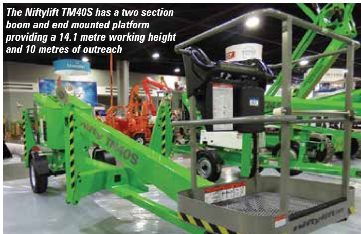
Niftylift exhibited an ultra-heavy duty straight telescopic trailer lift, the TM40S at the US Rental Show in February
