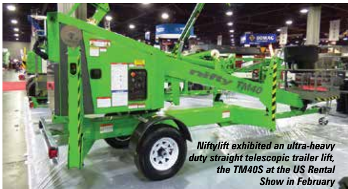
The Niftylift TM40S has a two section boom and end mounted platform providing a 14.1 metre working height and 10 metres of outreach
