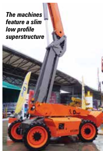
The new Dingli Italian booms use telehandler drive axles
