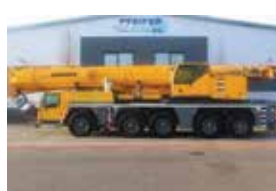
LIEBHERR - LTM1220-5.2 Telescopic Cranes
