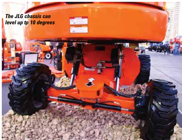
JLG showed a new Concept dynamic auto levelling boom at Conexpo last month
