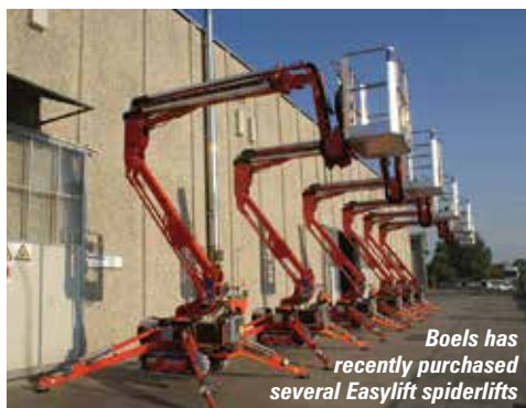
Spider lifts - due to their narrow stowed width and relatively high centre of gravity - are particularly prone to toppling over
