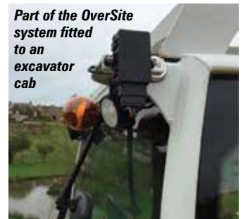
Wireless camera systems such as from BlockCam can easily be installed giving the operator a clear view of the working area from the cab
