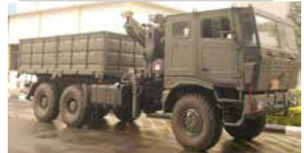
A 6x6 Tata truck complete with material handling crane for the Indian Army.
