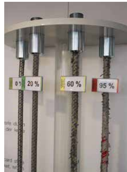
The different wear rates of the Liebherr Fibre rope.
