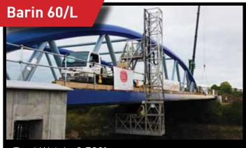
Total Weight **3,500kg**Vertical reach below bridge deck **4.0m**Horizontal reach under bridge deck **6.0m**Platform payload **300kg**Width taken up on bridge deck **2.0m**Underbridge platform rotation **180 degrees**
