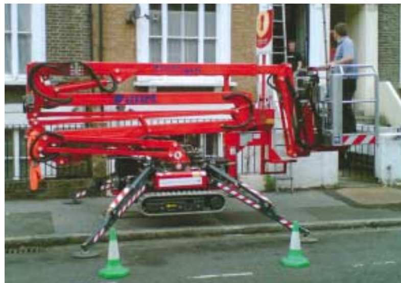
The units are well suited to urban situations, thanks to the ability to level themselves and their light weight.
