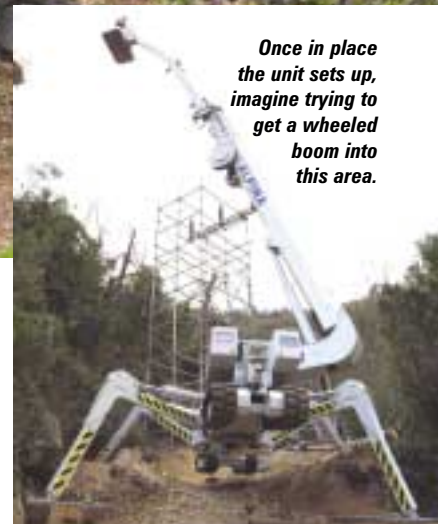
The 42m Falck-Schmidt, owned by Alpina, negotiates a heavily wooded mountain slope in France to reach transmission towers.
