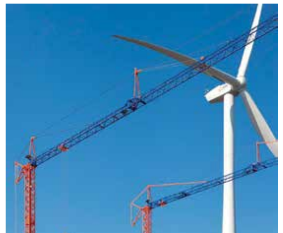
Arcomet's new crane has 8,000kg capacity, a 50 metre jib and maximum 36 metre hook height.
