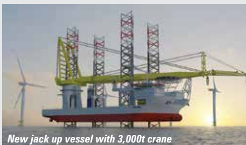
New jack up vessel with 3,000t crane
