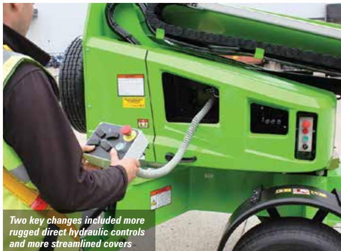
Niftylift's first straight telescopic aerial lift - the 14.1 metre TM40S trailer mounted lift
