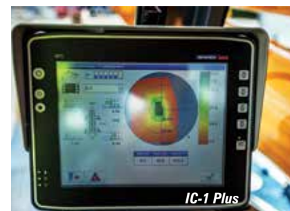
The outriggers have a new measurement system
