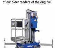
UpRight MX19 that helped kick off the micro scissor revolution back in 1994, although as with other machines in the size range it now weighs over 1.5 tonnes - 1,540kg to be precise - and has an overall stowed length of 1.85 metres. Overall width is 770mm, overall stowed height with guardrails up is 2.13 metres and platform capacity is 230kg with 115kg on the 900mm platform extension which extends the overall platform length to 2.54 metres.
