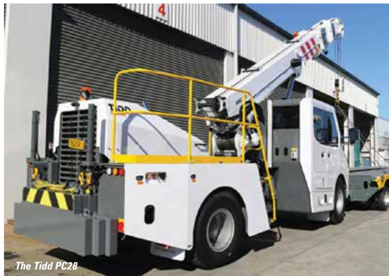
The Tidd PC28 features the new Slew Safe feature designed to minimise the risk of the crane toppling over when carrying a load on uneven surfaces
