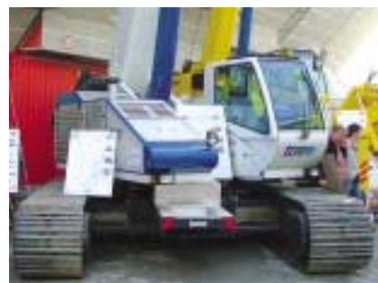
TCM showed several new telescopic crawlers, with and without outriggers. This RTC-50.2 has adjustable width tracks.
