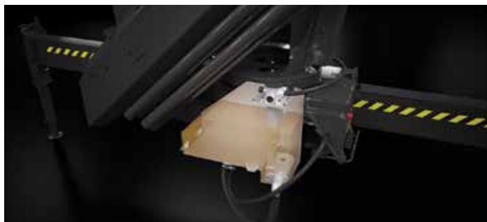
The new cyclone tank is a third of the size of a regular tank and effectively 'de-aerates' the returning oil.
