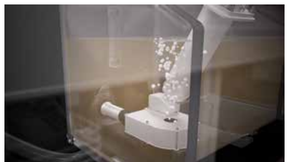
The new cyclone tank is a third of the size of a regular tank and effectively 'de-aerates' the returning oil.
