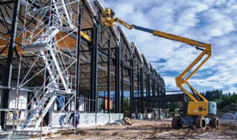
The HA20 LE has a small Stage V 'range extender' diesel engine that simply tops up the batteries
