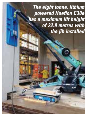
The Hoeflon C30e has a five section main boom topped by an optional five section telescopic luffing jib.
