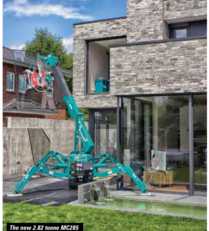
The new 2.82 tonne MC285 has load monitored multi-position outriggers
