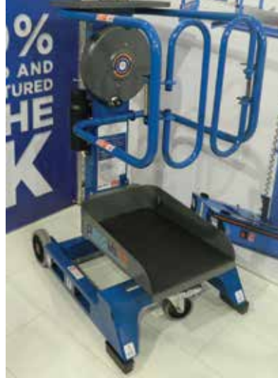
The Pecolift 1.2 with a maximum working height of 3.2 metres and a 150kg platform capacity weighs 117kg, has an overall width of 730mm, is less than a metre long and under 1.5 metres high stowed.
