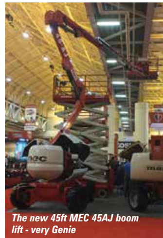
The MEC 45AJ features a two part right hand wrap around cover with greater protection during transport, better access and lower noise levels
