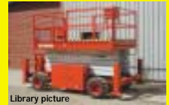
SNORKEL SL4084 (1998) Self propelled scissor lift. 4wd. 46' working height. Diesel. Repainted, serviced & tested.
