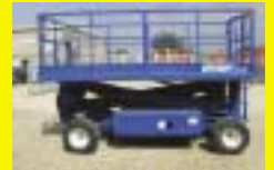
UPRIGHT SL26 (1990 & 1999) Choice of 2. Self propelled scissor lift. 32' working height. Diesel. 4wd Recently repainted, serviced & tested.
