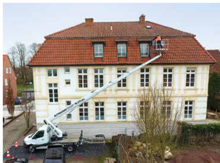
The Ruthmann TB270 pro offers up to 18.1 metres of outreach - 1.7 metres more than the previous model - while 15 metres is possible over the side.
