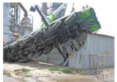
Overturns are almost always caused by operator error.
