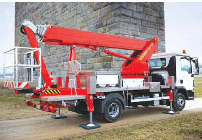
The Palfinger P 280 CK is mounted on a 7.5 tonne chassis with a maximum outreach of 18.8 metres and 300kg platform capacity.
