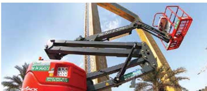
Skyjack S46AJ articulated boom lift.
