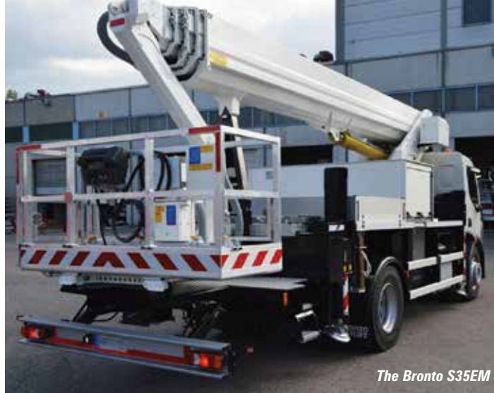
The Bronto S35EM has a maximum outreach of 29 metres and maximum platform capacity is 500kg
