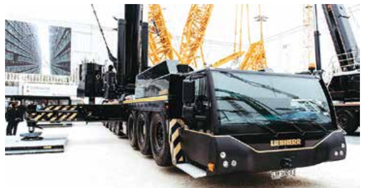
The LTM 1650-8.1 has an 80 metre main boom but to keep within the 12 tonnes per axle transport weight it can be specified with a 54 metre boom and removeable rear outriggers.
