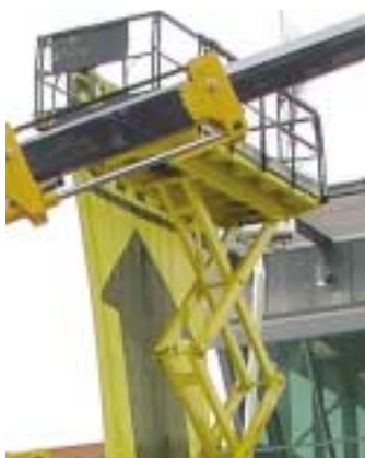
It is light but large objects that cause the most danger to a scissor lifts stability, such as this huge banner.
