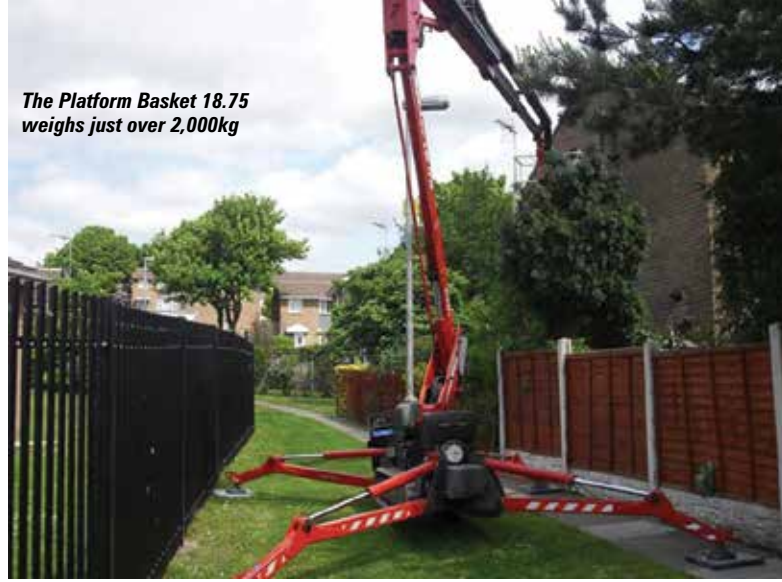
The new Klubb K21B uses battery power for the work platform
