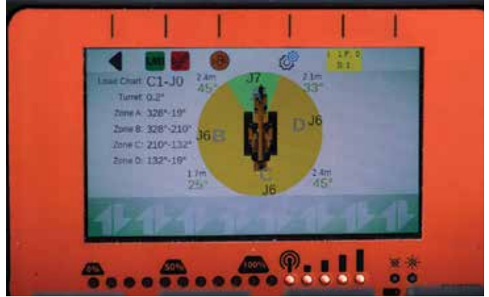
The remote controllers display screen contains all the information, needed including actual outrigger set-up and slew position.
