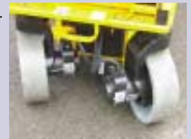
The JLG was the only unit with direct electric front drive.
