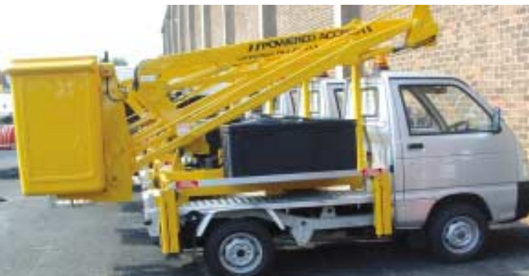
A completed shipment of 11 metre lifts on Piaggio Porter chassis
