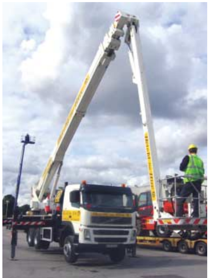
Ireland's largest truck mount 50m Bronto 55MDT owned by Easi-UpLifts
