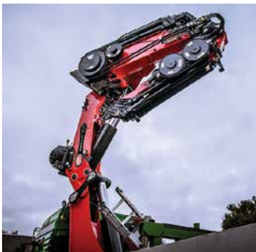
The HMF 7020 K8-RCS can take 2,050kg to 20.4 metre radius.
