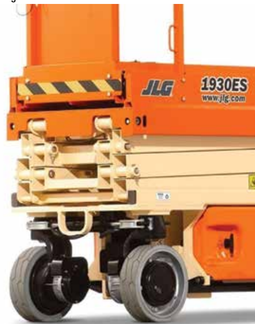
JLG 1930ES front axle electric drive.
