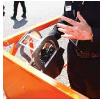
Snorkel Guard secondary guarding system covers the lift control box which when pressed stops the machine rising.
